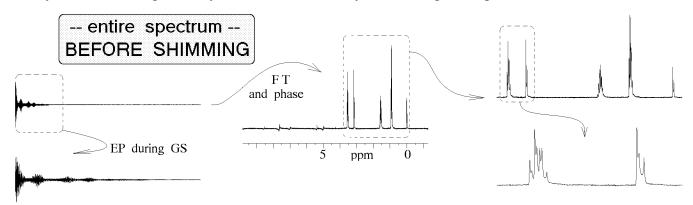
The main advantage of monitoring the FID of a *single, sharp* NMR line rather than the FID of an entire spectrum is that the envelope should be a simple, decaying exponential. You can be sure that any deviations from this ideal shape must arise from the magnetic field gradients which you are trying to cancel with the shims.
