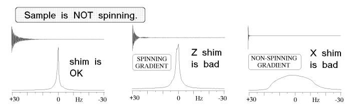
EFFECT OF SAMPLE SPINNING: Distortions of the FID and of the lineshape which are caused by spinning gradients are not changed, but distortions caused by non-spinning gradients are greatly reduced. Some of the third-order non-spinning gradients cannot be shimmed out on the WM-360, and they cause the base of the NMR line to broaden slightly when the spinner is stopped.
